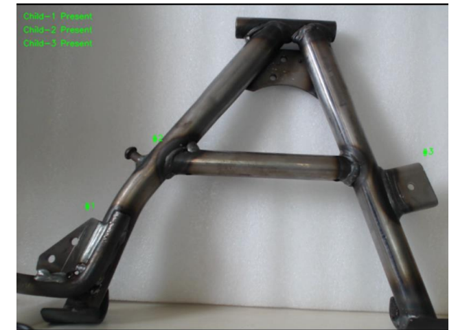
Detecting presence of all child parts and the welding quality for brake pedal
